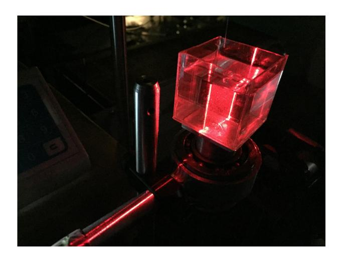
A sheet laser illuminates a toroidal droplet formed in silicone oil to help researchers image the flow field movement inside the droplet. Credit: John Toon, Georgia Tech
