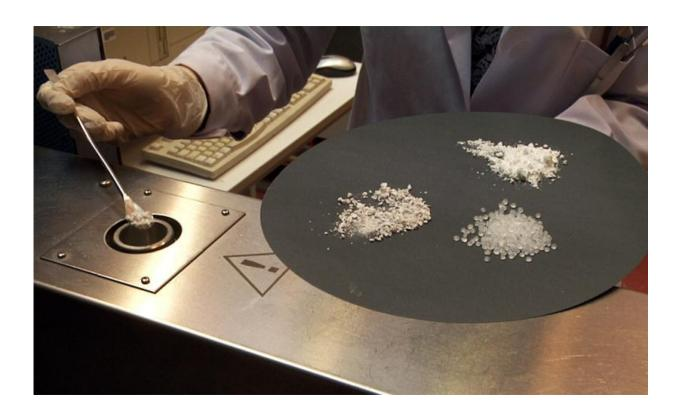
Materials used for the manufacture of the ceramic electrodes of the batteries. Credit: Universidad Carlos III de Madrid
