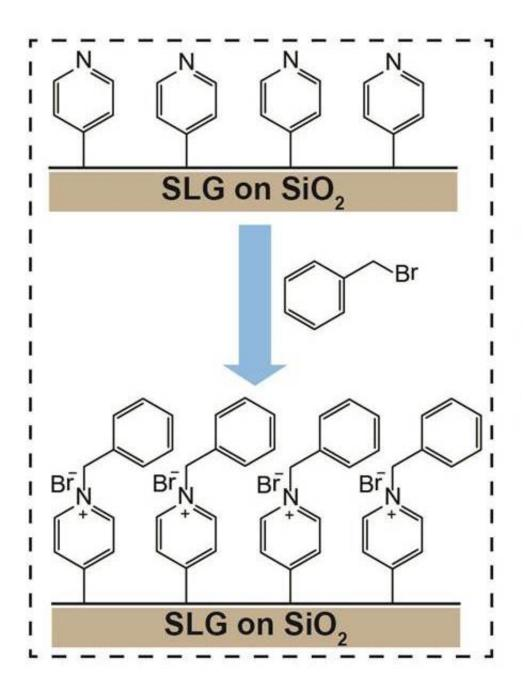
Figure 3: Functionalized graphene allows additional functionalization.A schematic diagram showing the reaction between 4-pyridyl groups that were decorated on single layer graphene (SLG) and benzyl bromide. This sequential functionalization expand the applications of graphene. Credit: Institute for Basic Science
