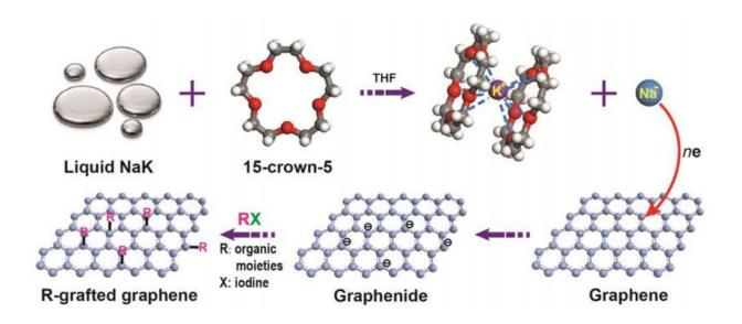
Graphene's functionalization reaction. The sodium-potassium alloy (NaK) in solution forms a sodium ion (Na-) when it meets the crown ether molecule (15-crown-5). Na- reduces graphene and makes it more reactive towards other molecules (R). The "decorated" graphene has several potential applications. Credit: Institute for Basic Science
