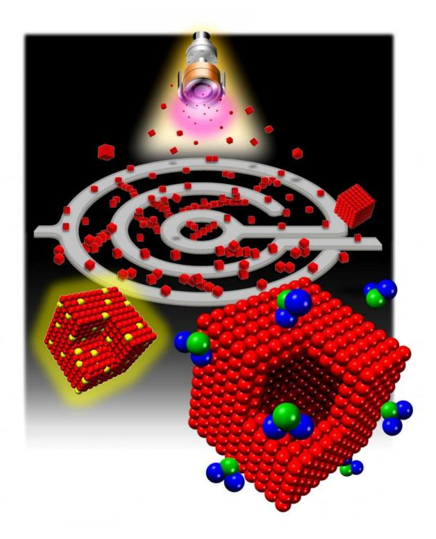
This schematic depicts the production of iron nanocubes using magnetron-sputtering inert-gas condensation and the use of these cubes in NO2 sensors. Credit: Okinawa Institute of Science and Technology
