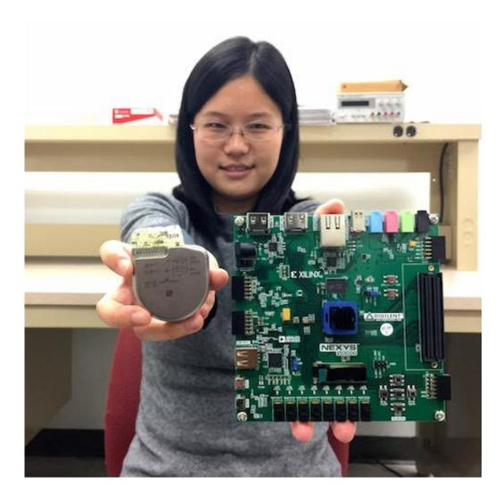
UA doctoral student Sixing Lu is helping ECE associate professor Roman Lysecky develop technology on a prototype network-connected pacemaker (in left hand) to detect hacking of a real pacemaker (in right hand). Credit: UA College of Engineering
