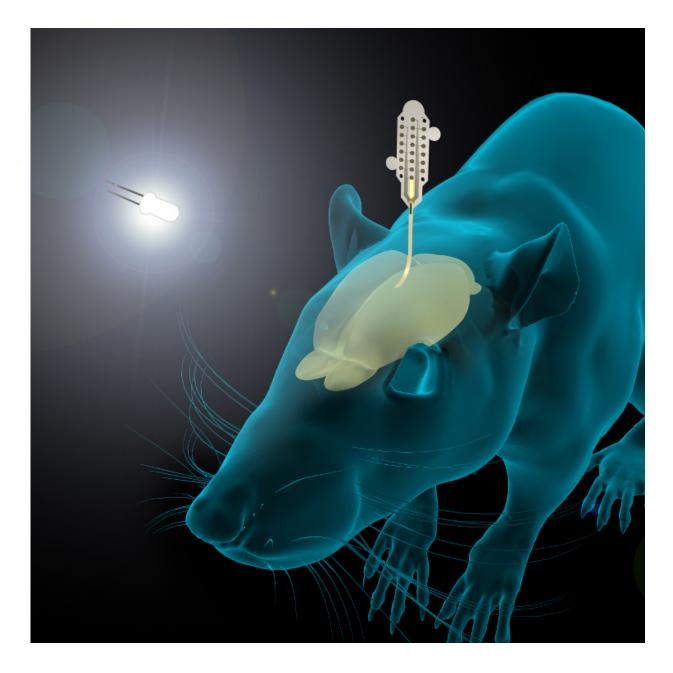
The graphene-based neural probes were used to detect rats' responses to visual stimulation, as well as neural signals during sleep. Both types of signals are small, and typically difficult to measure. Credit: ICN2
