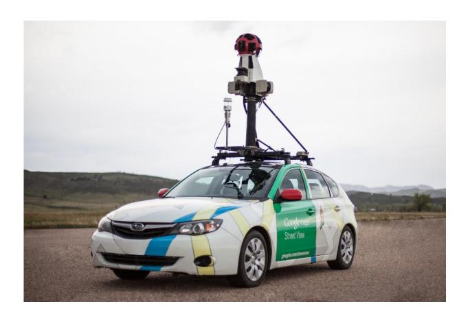
Some Google Street View cars have been specially equipped with methane analyzers to detect methane lakes from natural gas lines. Credit: EDF
