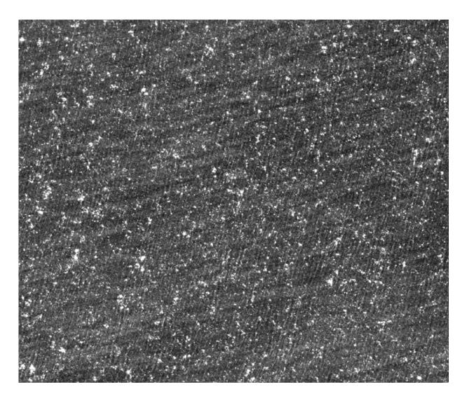
Sun glitter patterns measured by Sentinel-2A in the western Mediterranean Sea in Band. Surface swell waves are seen in a roughly north–south orientation with bright areas showing large breaking waves. The wind was very strong (about 20 m/s) blowing from the west. Dark patches in the image are areas of flows leading to calmer waters and reduced Sun glitter. Credit: contains modified Copernicus Sentinel data (2016), processed by ESA
