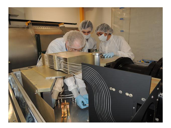
Three instrument team members work on the APOGEE South instrument, before the top was closed. It was then cooled down and placed under vacuum ready for observing. Left to right: Garrett Ebelke, Matt Hall, and Mita Tembe (all from the University of Virginia). Image Credit: John Wilson (University of Virginia)
