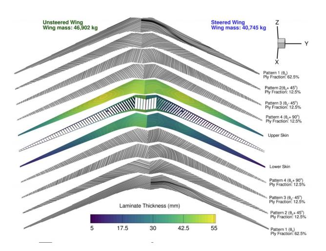
Tow-steered composites can reduce the structural weight of an aircraft by 10 percent while reducing fuel burn by 0.4 percent. NASA is building a prototype of a tow-steered wing box for a scale test at the Armstrong research center. Above, a variety of tow-steered designs developed by Martins. Credit: Joaquim Martins, Timothy Brooks (UM) and Graeme Kennedy (Georgia Tech)
