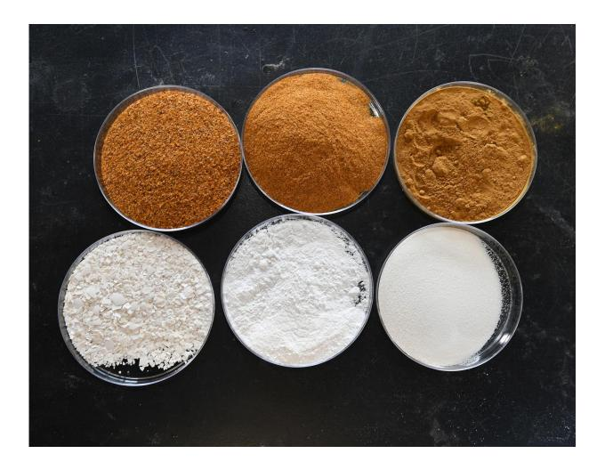
Researchers at The Ohio State University have developed a patent-pending technology for incorporating food waste into rubber. Here, dried and ground tomato skins (top) and eggshells (bottom) are shown after coarse, medium, and fine processing before being added to rubber. Credit: Kenneth Chamberlain, The Ohio State University.
