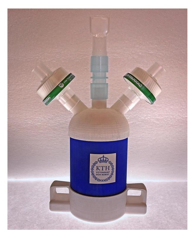
Highly-charged needles inside the bottle ionize the micro-sized droplets of water that carry the virus in the breath. Credit: KTH Royal Institute of Technology
