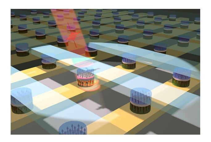
One modification researchers made to the device was to use a transparent electrical material called indium tin oxide for the electrode to allow light to pass through it. These layers are stacked into a pillar with a diameter of only 10  $\mu m$ , which is only one-tenth the diameter of a typical human hair. Credit: Junyang Chen, University of Minnesota
