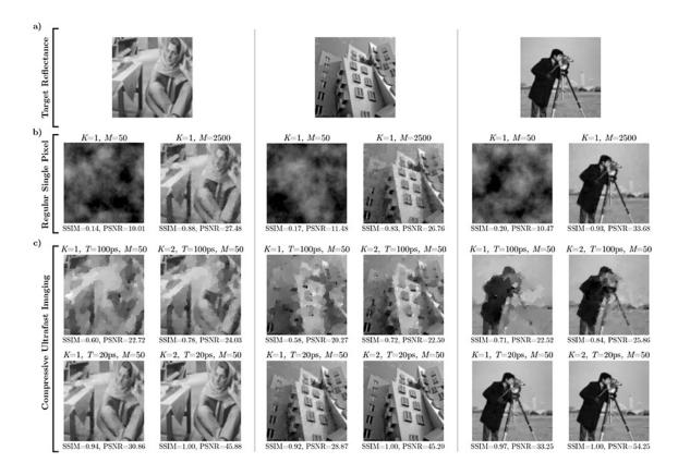
Researchers from the MIT Media Lab developed a new technique that makes image acquisition using compressed sensing 50 times as efficient. In the case of the single-pixel camera, it could get the number of exposures down from thousands to dozens. Examples of this compressive ultrafast imaging technique are show on the bottom rows. Credit: Massachusetts Institute of Technology
