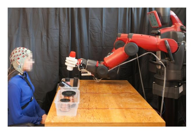
A new feedback system enables human operators to correct a robot's choice in real-time. Credit: Jason Dorfman/MIT CSAIL
