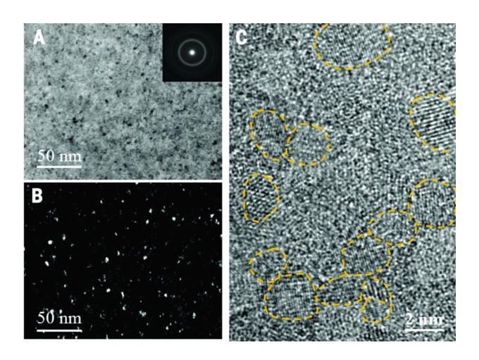
Microstructure of the as-deposited nanograined Ni–Mo alloy. (A) Bright-field and (B) dark-field images of the as-deposited Ni–21.5% Mo sample. (Inset) A corresponding selected area diffraction pattern. (C) A HRTEM image of the same sample showing individual grains outlined by dashed lines. Credit: (c) *Science* (2017). DOI: 10.1126/science.aal5166
