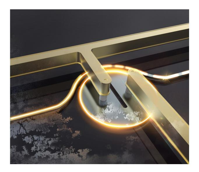
An illustration of a silicon photonic micro-disk modulator operating at cryogenic temperatures. Light traveling down the silicon waveguide couples to the resonance of the micro-disk cavity. An electrical signal applied to the disk shifts
