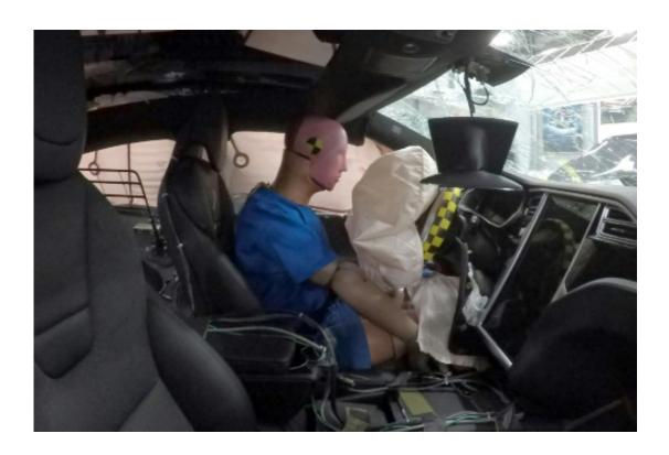
A technology-packed, 180-pound (80 kg) crash test dummy sends a vast array of data from its sensors to show how he fared in the crash
