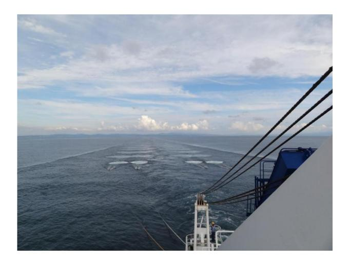
The wake behind this JAMSTEC research vessel is caused by the seismic sensors being towed behind the boat. The sensors allow researchers to create detailed images of the bedrock and structures under the ocean's bottom. Credit: JAMSTEC
