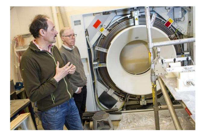
Martin Landrø (left) shown here with his colleague Ole Torsæter, has used a variety of tools to study subsea geology. Here he is shown with an x-ray machine used to examine sandstone from oil reservoirs. Credit: Ole Morten
