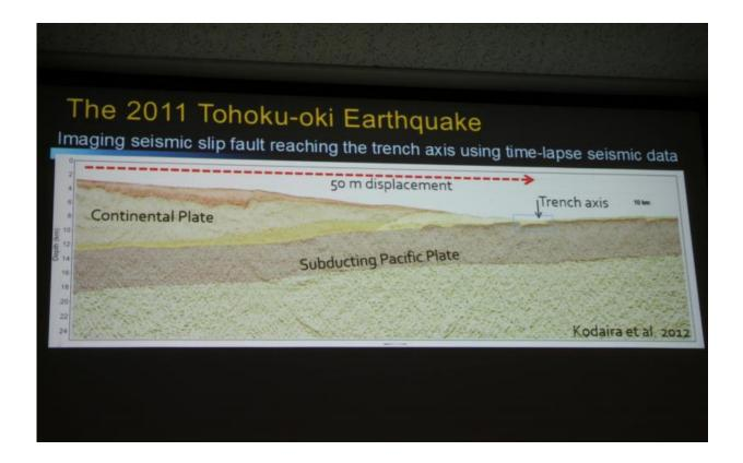
Here's an example of the kinds of images that are produced of the geology below the seafloor using seismic data to create an image. Credit: Anne Sliper Midling, NTNU
