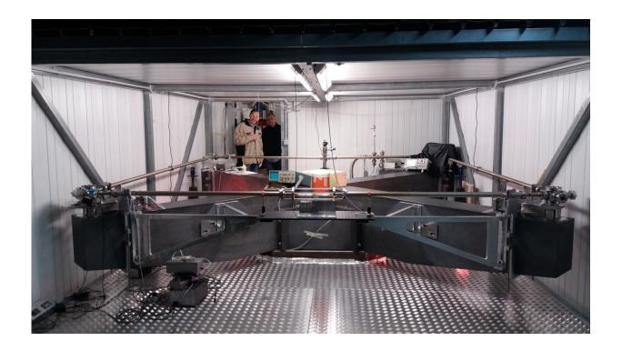
The GINGERino ring laser gyroscope, which is a square cavity with a side length of 3.6 meters. Credit: Belfi et al.
