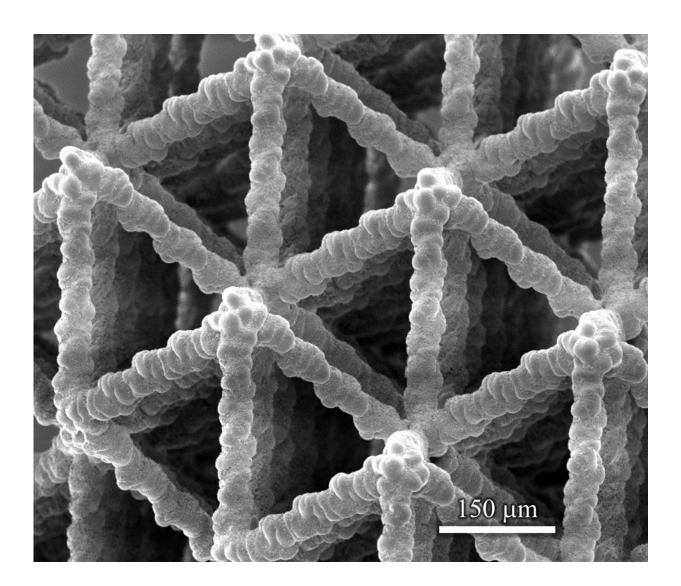
Microstructures like this one developed at Washington State University could be used in batteries, lightweight ultrastrong materials, catalytic converters, supercapacitors and biological scaffolds. Credit: Washington State University
