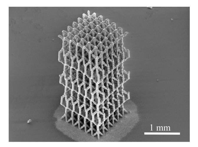
Microstructures like this one developed at Washington State University could be used in batteries, lightweight ultrastrong materials, catalytic converters, supercapacitors and biological scaffolds. Credit: Washington State University
