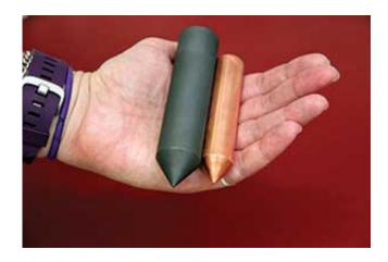
Ames Laboratory scientist Deborah Schlagel holds a graphite crucible (left) and a Bridgman-grown copper crystal (right). Credit: Ames Laboratory
