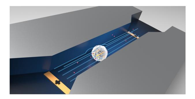
3-dimensional rendering of a cell passing through the electroporation zone while a pulse is being applied. The electric field lines which normally do not penetrate an insulating cell are able to penetrate the cell through the conductive pores. Credit: *Technology Journal*
