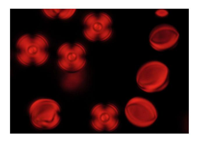
A magnified image of liquid crystals confined to spherical tactoids. Credit: Georgia Tech
