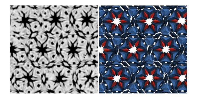
Left: An electron microscope image of a slice of the crystal structure. Credit: Mirkin Lab, Northwestern University. Right: A matching slice from a simulation of the crystal structure. Credit: Glotzer Group, University of Michigan. Copyright: Science
