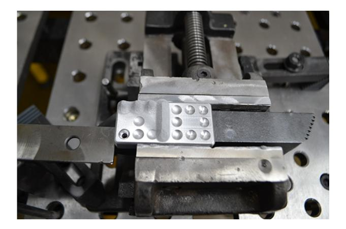
This aluminum domino is a before/after demonstration of how the Supersonic Particle Deposition (SPD), also known as Cold Spray, applies metal particles to a worn part, building up and repairing surface damage. Credit: University of Akron
