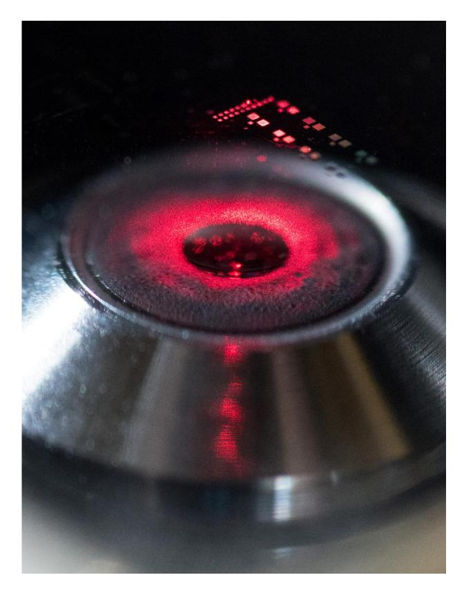
Laser light shows the nanopatterned structure of a chiral metamaterial developed
