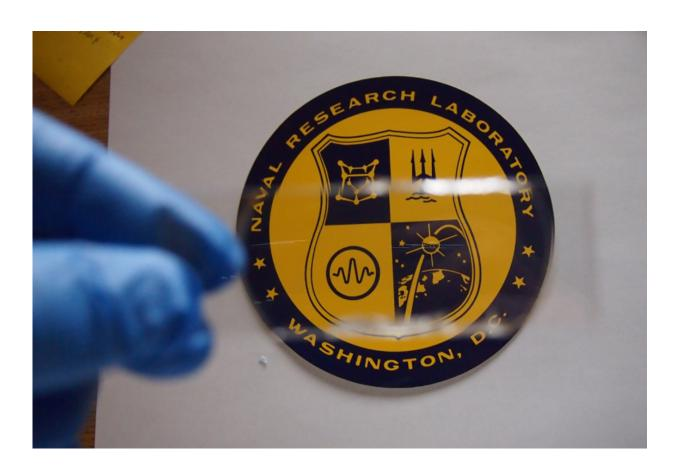
The NRL-developed transparent polymer armor consists of alternating layers of elastomeric polymer and a harder material substrate. Very small crystalline domains, which also provide rigidity, give the polymer its transparency. Credit: U.S. Naval Research Laboratory
