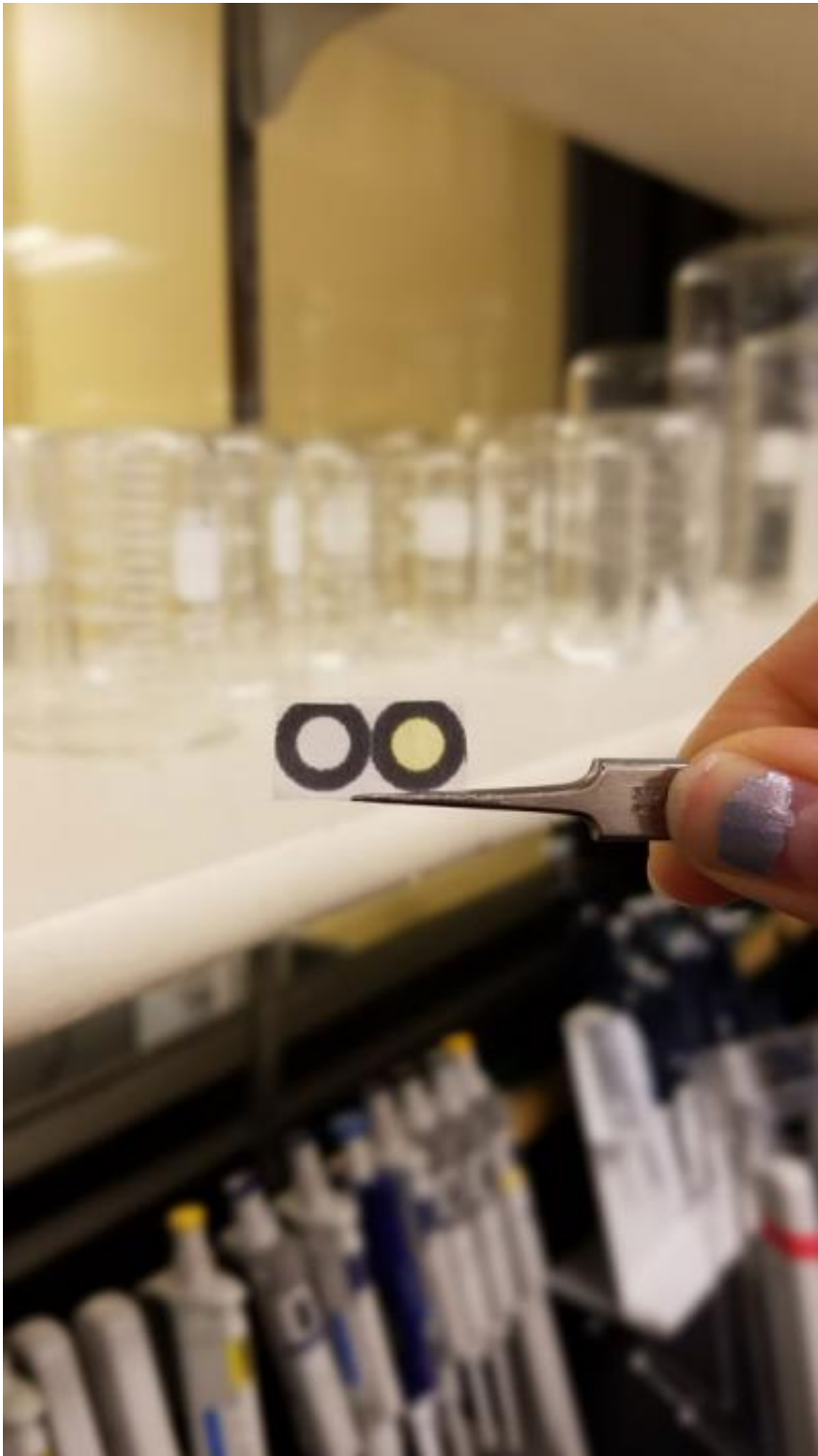
A paper-based colorimetric test strip that can detect harmful bacteria. Credit: Henry Lab/Colorado State University
