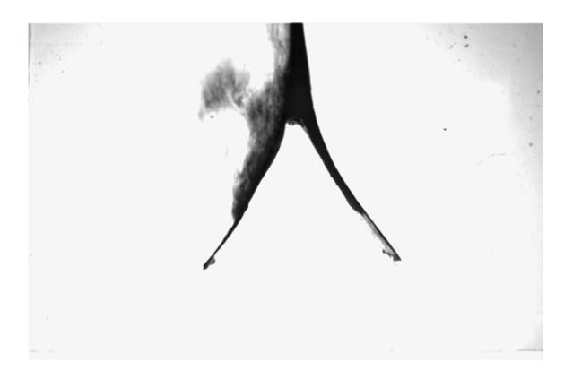
Alternate boiling on two heater circuits swings the apparatus in liquid coolant. Credit: UIC/Alexander Yarin
