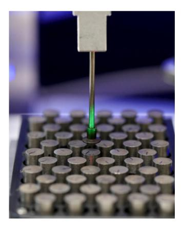
A second generation of the Pu-238 pellet automated metrology system being developed in an ORNL lab. Credit: Oak Ridge National Laboratory
