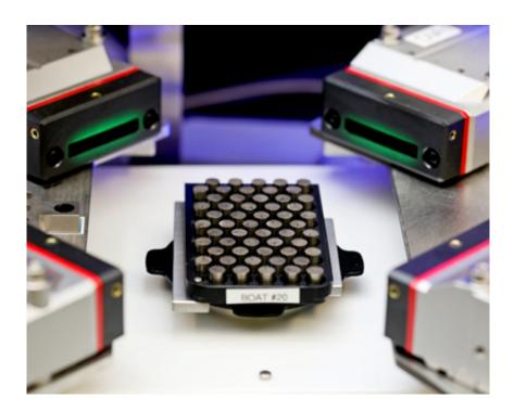
A second generation of the Pu-238 pellet automated metrology system being developed in an ORNL lab.
