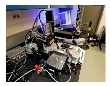
A second generation of the Pu-238 pellet automated metrology system being developed in an ORNL lab. Credit: Oak Ridge National Laboratory
