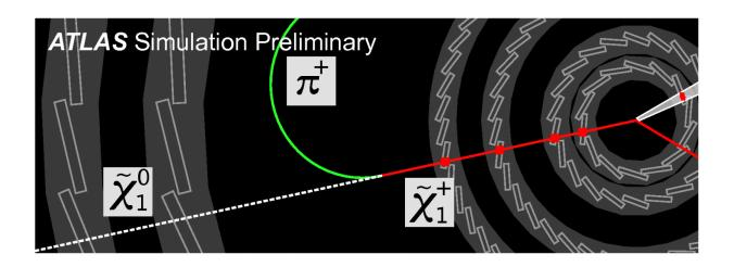
ATLAS simulation showing a hypothetical new charged particle ( $\chi$ 1+) traversing the four layers of the pixel system and decaying to an invisible neutral particle ( $\chi$ 10) and an un-detected pion ( $\pi$ +). The red squares represent the particle interactions with the detector. Credit: ATLAS Collaboration/CERN
