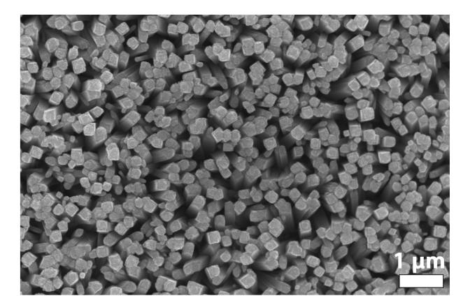
A photo shows an array of titanium dioxide nanorods with an even coating of an iron, manganese and phosphorus catalyst. The combination developed by scientists at Rice University and the University of Houston is a highly efficient photoanode for artificial photosynthesis. Credit: Whitmire Research Group/Rice University
