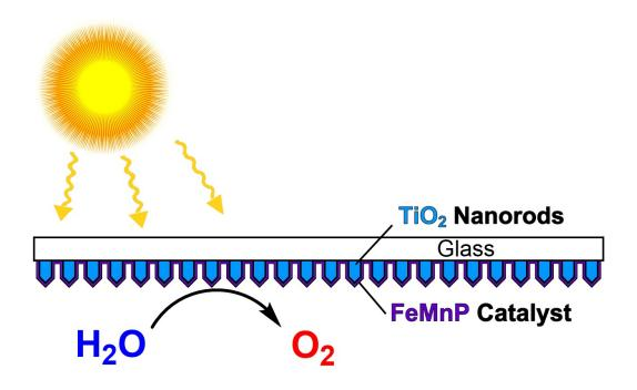
Scientists at Rice University and the University of Houston created a catalyst from three elements -- iron, manganese and phosphorus -- and then coated it evenly onto an array of titanium dioxide nanorods to create a highly efficient photoanode for artificial photosynthesis. Credit: Whitmire Research Group/Rice University
