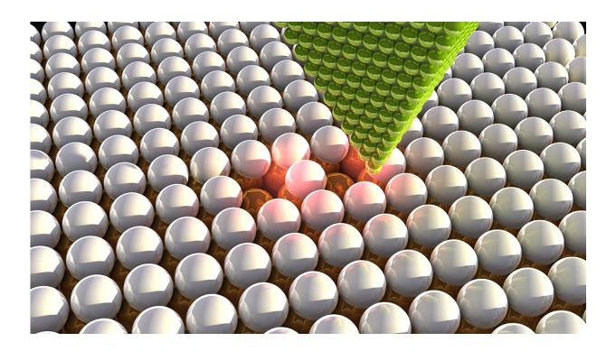
The tip of a scanning tunnelling microscope (STM) above chlorine atoms that have been deliberately moved. By moving individual atoms under their microscope, scientists were able to arrange vacancies in a single layer of chlorine atoms and create atomic lattices with a predetermined electrical response. Credit: Ella Maru Studio & Aalto University
