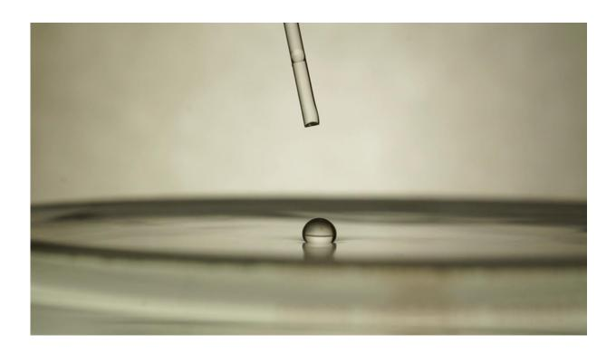
A 2-mm diameter acetone droplet in the Leidenfrost state on a 70 C water bath. Credit: Stoffel D. Janssens
