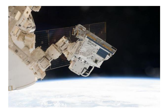
The STP-H5 palette of instruments being maneuvered by the robotic arm on the International Space Station. The Cornell antenna array is visible just to the right of the "Canada" logo. This photo was taken during the installation process. Credit: NASA Johnson Spaceflight Center/Provided
