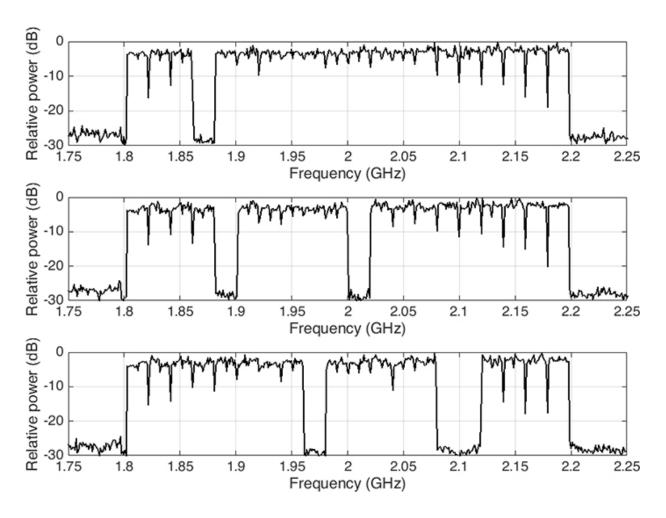
The new transmitter enables flexible specification of carrier waves in a wide frequency band of 400 MHz. Credit: Aalto University
