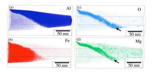
A new study evaluates the atomic behavior of metals during solid state welding and finds the resulting oxide film is dissolved near the material's surface. Credit: Oak Ridge National Laboratory
