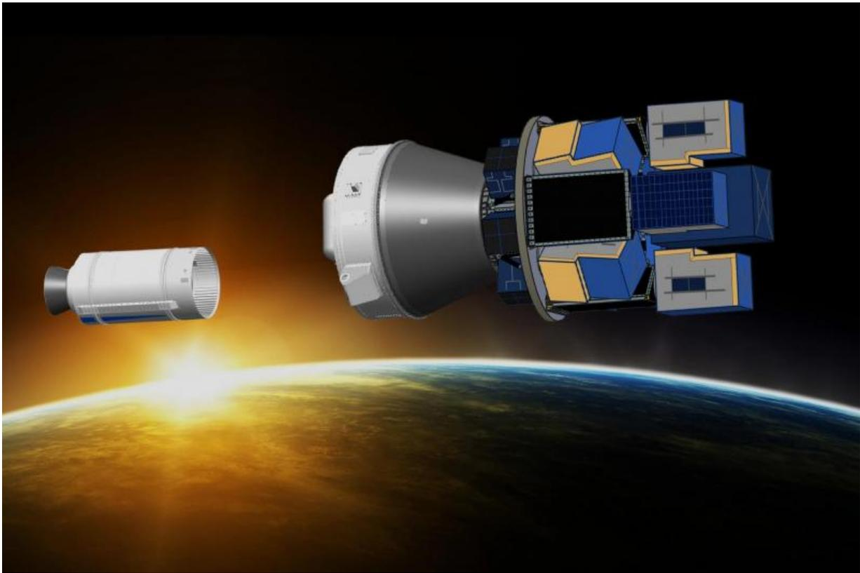
Europe's Vega small launcher is set to demonstrate its extended capability to deploy multiple light satellites using its new versatile Small Satellites Mission Service (SSMS) dispenser, in the second half of 2018. Credit: ESA
