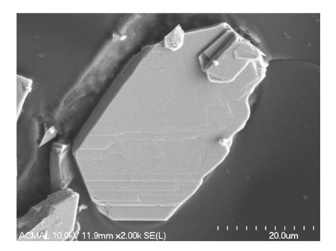
A scanning electron microscope reveals the distinct shape of leoszilardite crystals. Credit: Travis Olds
