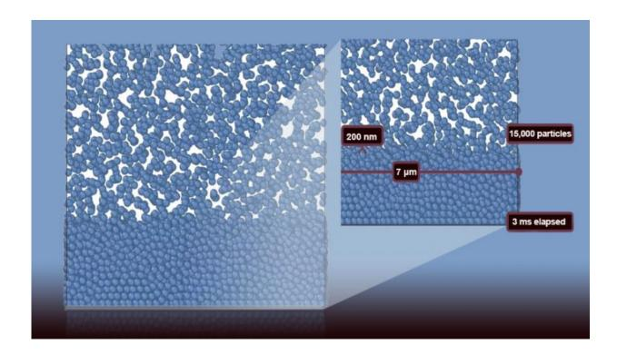
The new electrophoretic deposition model developed at Lawrence Livermore tracks every single particle during the entire EPD process, each particle being roughly the diameter of the smallest bacteria. Credit: Lawrence Livermore National Laboratory
