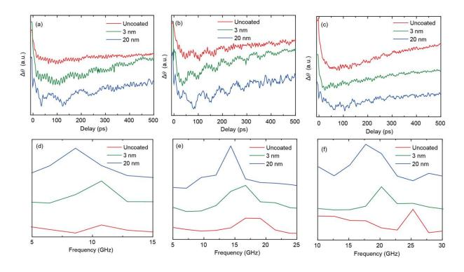
Transient Kerr rotation signals of the uncoated LSMO film and the LSMO films coated with 3- and 20-nm-thick BFO layers under external magnetic fields of 0.2 T (a), 0.4 T (b), and 0.6 T (c). The Fourier transforms of the signals shown in (a), (b), and (c) for external magnetic fields of 0.2 T (d), 0.4 T (e), and 0.6 T (f), respectively. Credit: ©Science China Press
