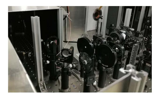
A time-resolved magneto-optical Kerr effect measurement system. Credit: ©Science China Press
