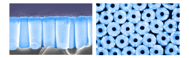
SEM images of a nanotube array: side view (left) and top view (right). Credit: UC San Diego Jacobs School of Engineering
