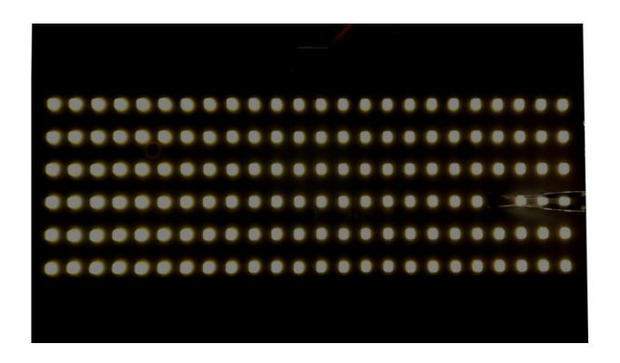
Array of low-power light-emitting diodes. Failure of a single LED does not affect the overall system. Credit: Karlsruhe Institute of Technology
