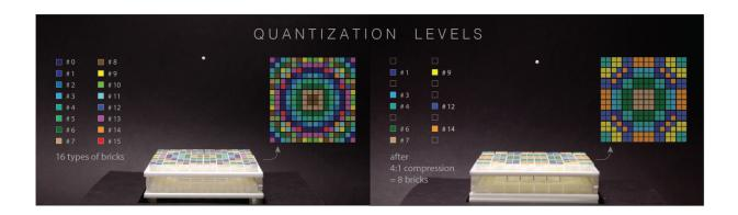
Slightly different metamaterial bricks are combined to create any desired acoustic field. Credit: Interact Lab, University of Sussex
