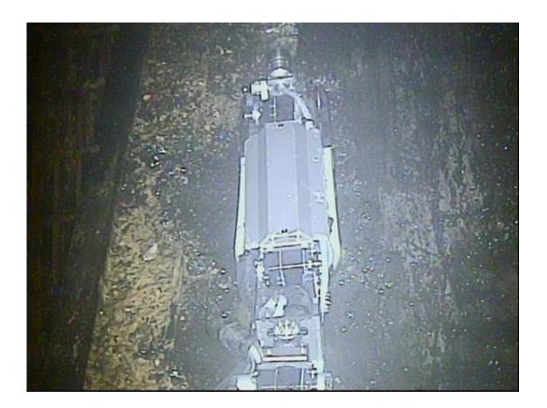
This Feb. 16, 2017 photo released by Tokyo Electric Power Co. (TEPCO) shows a remote-controlled "scorpion" robot inside the Unit 2 reactor's containment vessel at Fukushima Dai-ichi nuclear power plant in Okuma town, Fukushima prefecture, northeastern Japan. Robot probes sent to one of Japan's wrecked Fukushima nuclear reactors have suggested worse-than-anticipated challenges for the plant's ongoing cleanup. (TEPCO via AP Photo)
