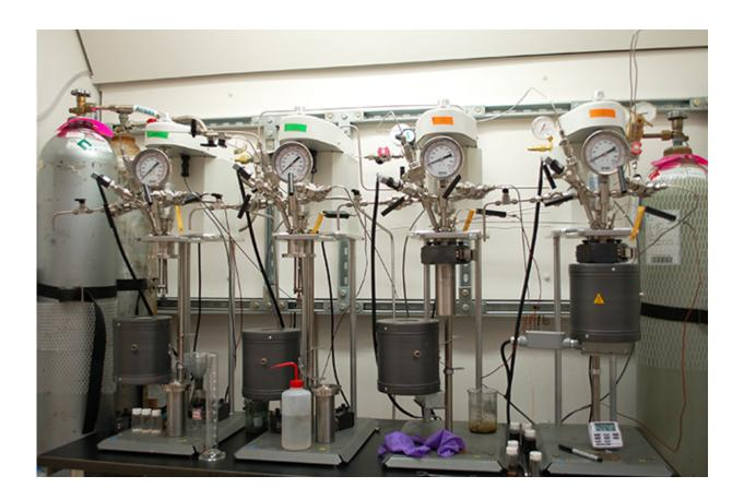
Catalytic conversion of biomass-derived chemicals to renewable polymers occurs in laboratory stirred-tank reactors. Credit: University of Minnesota
