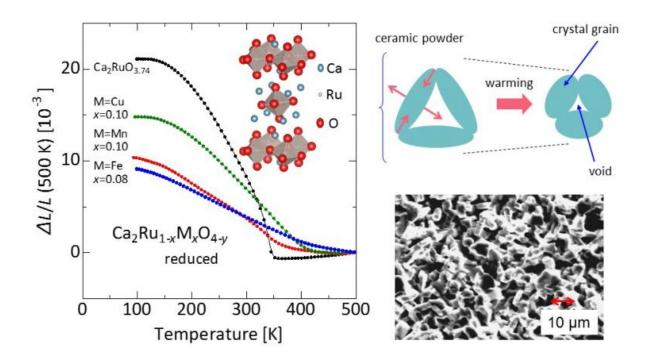
A layered ruthenate Ca2RuO4-y ceramic body contracts on heating, or exhibits negative thermal expansion (NTE). The sintered-body structure shows colossal NTE when extremely anisotropic thermal expansion of the crystal grains produces deformation, consuming open spaces (voids) on heating. The total volume change related to NTE reaches 6.7% at most, the largest reported so far. Credit: Nagoya University
