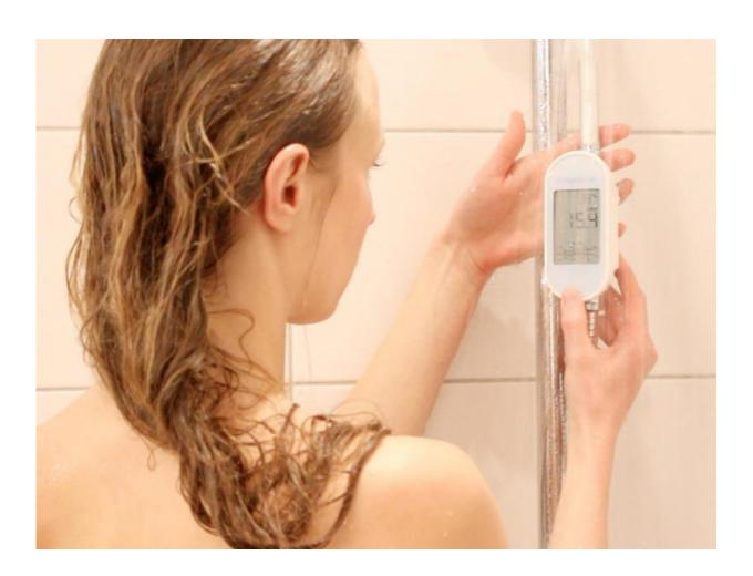
The measuring devices are fitted below the shower head. They allow water consumption, water temperature and energy use to be seen at a glance. Credit: Liliane Ableitner/Universität Bamberg
