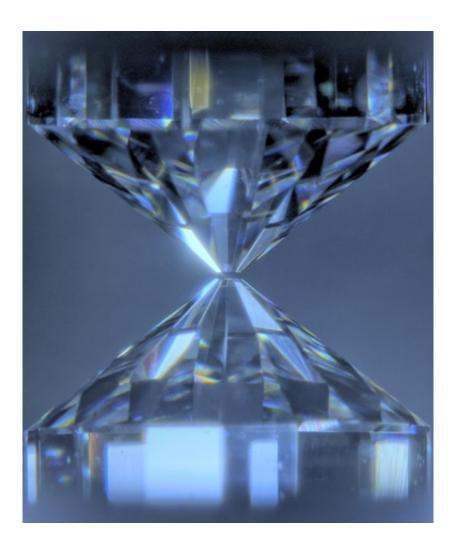
The samples are heated under pressure to high temperatures of the core (about 4000 kelvins and higher) by being irradiated by a laser through diamonds. Credit: Tokyo Institute of Technology
